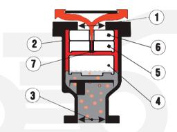
Disentrained air rises through the liquid and accumulates in the valve chamber. When the volume of air is sufficient to displace the liquid, float (4) will no longer be buoyant and will gravitate downwards thereby opening the small orifice (7) and allowing accumulated air to be discharged into atmosphere. As air is discharged the liquid raises the float (4) and re-seals the small orifice (7) and prevents the escape of liquid.
