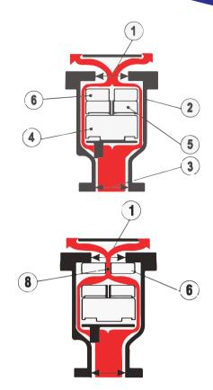
3. **Pressurised air release from a full pipeline** Subsequent to the filling of a pipeline, liquid enters the valve barrel chamber (2) and the floats (4), (5) and (6) are buoyed so that the large orifice (1) is closed by float (6). The valve will then become internally pressurized. A minimal working pressure of 0.5 bar (7.3 psi) acting on the relatively large area of the orifice (1) will lock float (6) into the closed position across the large Orifice (1).
